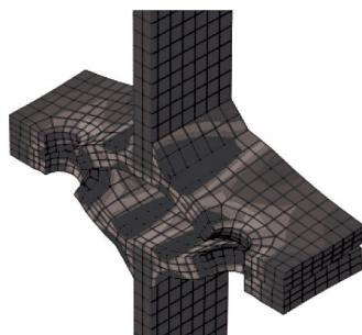
**Figure 10.** Plastic hinges development in numerical models
