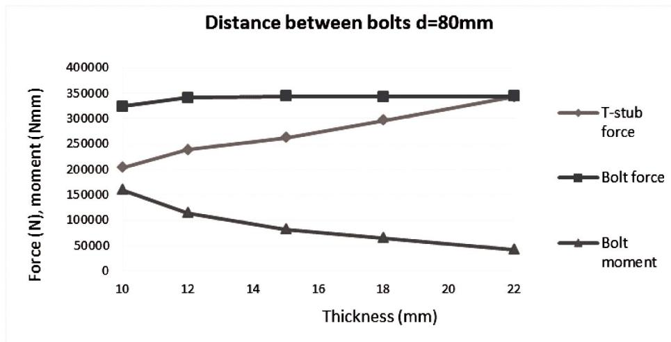
**Figure 18.** Variation of T-stub force and bolt forces with increasing thickness of end plate
