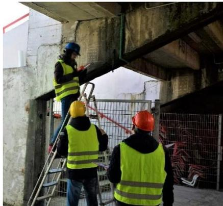
**Figure 21.-Schmidt hammer testing process**
