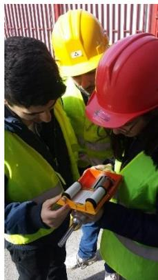
**Figure 22.-Schmidt hammer testing process**
