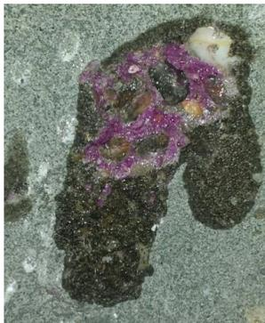
**Figure 25.-** Phenolphthalein test GN 10-11
